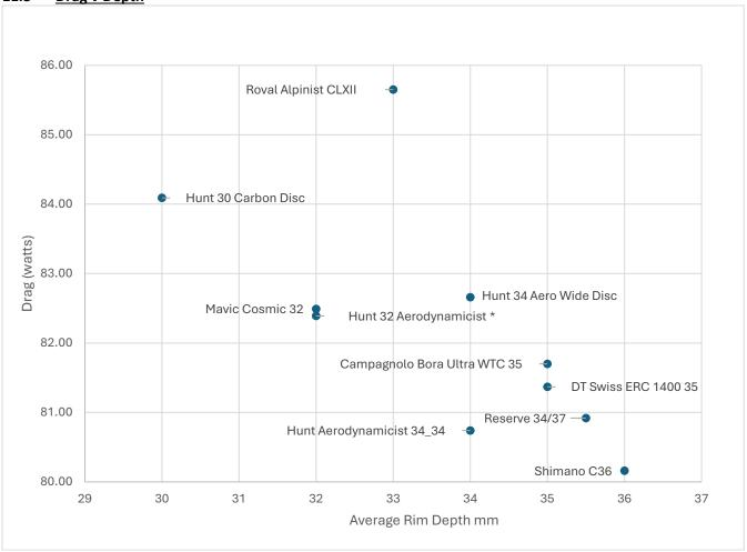
The Shimano Dura-Ace C36 achieved the drag reduction through increased rim depth with an increase in weight.
