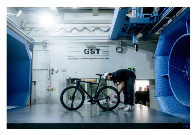
The GST Windkanal was used for this project. GST is a low-speed open wind tunnel constructed in 1986 for use by Airbus Space and Defence and is well suited for bicycle testing – used and recognised widely in the cycling industry for independent product development testing.
