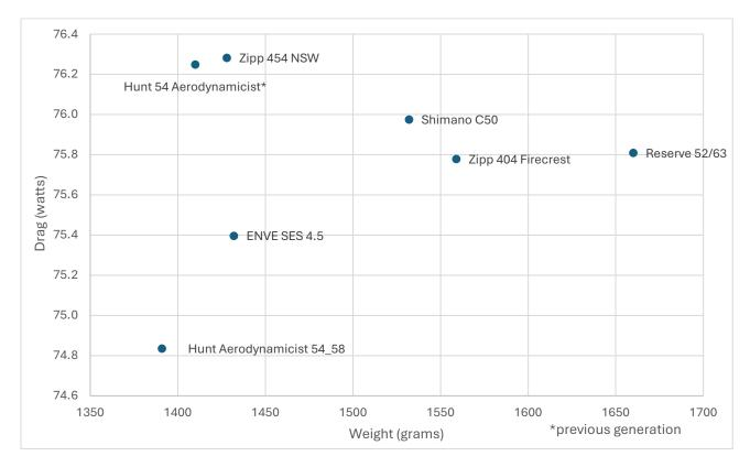
The Hunt Aerodynamicist 54\_58 was the clear leader when considering the combination of weight and low drag.
