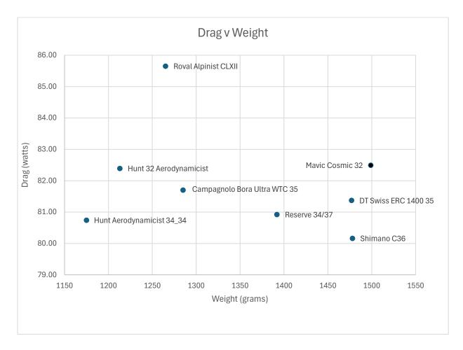
The aim with this wheelset was to produce a shallow section wheel with excellent aerodynamic performance, but at a weight that would enable it to be used as a mountain climbing wheel. The only competitor wheel that was faster than the new Aerodynamicist 34\_34 was the Shimano Dura-Ace C36, which carried a weight penalty of over 178grams per wheelset, this for a drag reduction of only 0.58 watts.
