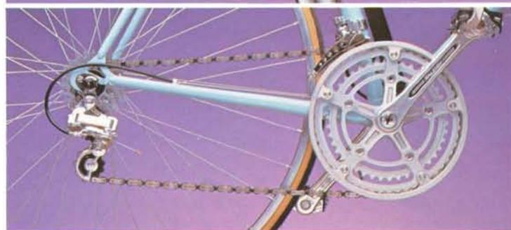
PRO-AM equipped with 12-speed transmission. Sun Tour alloy VX gear using Ultra 6 chain and freewheel block.
